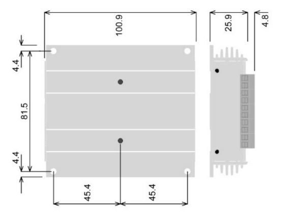
The DLC-C2P6-D-E can be mounted from above using the M4 clearance corner holes, or from beneath using the M4 tapped holes (maximum screw length inside is 6mm).
